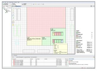
Data Center Operation for Colocation extends the usage of DCIM tools to the multi-tenant sales process, where it provides instant visualization of space available for selling on to tenants, broken down by used, reserved and available capacity, and identifies how much is required going forward. This expands the user group of DCIM into the front office of the business - making it a driver for
